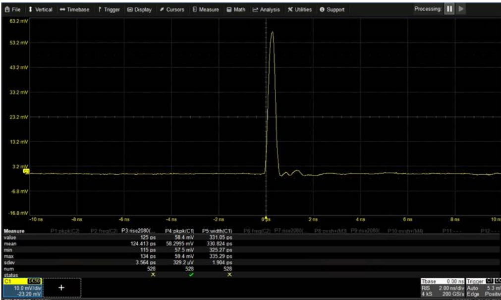
5. AWG-5000 | Pulse wave | 140 mVpp Amplitude | Attenuator 30 dB | Oscilloscope
